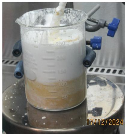
Fig. 14: *Bismuth trioxide suspension after precipitation with concentrated NaOH*
