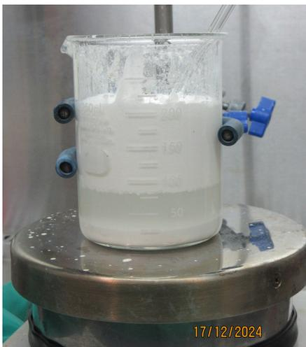
Fig. 13: *Bismuth trioxide suspension before precipitation*
